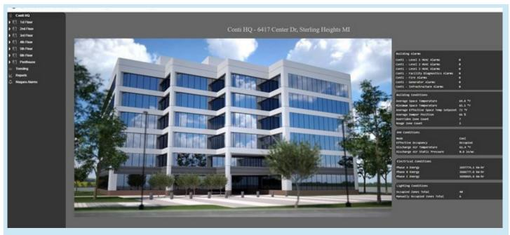
Example of a Conti-developed home screen for a large building. The graphical user interface (GUI) needs to provide for easy navigation from the portfolio-level, to floor-level, down to pieces of equipment and even VAVs. Visualizations are designed for easy, unambiguous interpretation to facilitate quick reaction and resolution of alarms.
