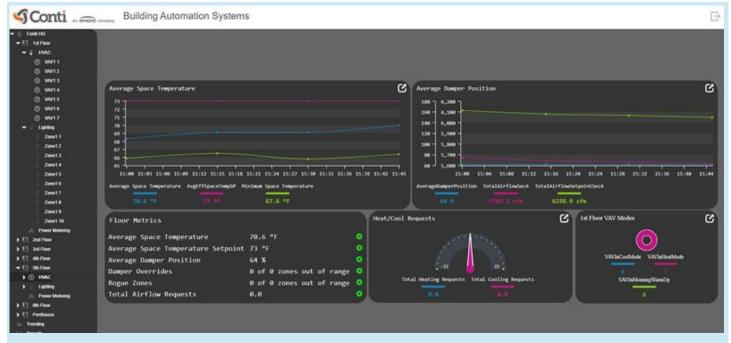
Floor-level metrics allow a secondary evaluation of floor-level conditions, easily identifying any deficiencies in floor-level units or the upstream units serving the floor. From one graphical page, the end user can determine mode, operation and operator overrides that could negatively influence the space.
